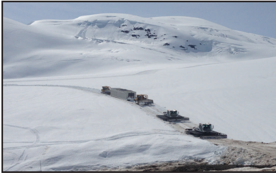
WWTP being transported to the top of the glacier.
